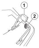
3 Select the required cutting height (1-10) with the cutting height lever.
