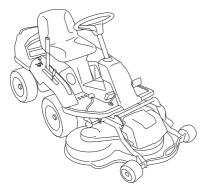
The power transmission from the engine is handled by a hydrostatic transmission, which allows variable variation of the speed by using the pedals.
