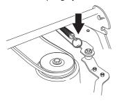
6 Lift off the drive belt and hang on the load-relieving hook.
