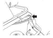
7 To secure the cutting deck from spring back, place a wooden block between equipment frame and chassis.
