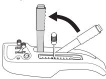
2 Move the throttle to the idle position. Turn the ignition key to the "STOP".
