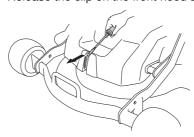
3 Loosen on the cutting height stay and place in the holder.
