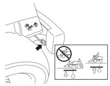
Pull out the control to disengage the drive system.
