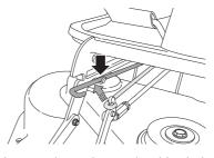
4 Loosen the spring on the drive belt's belt idler by pulling the spring eye.
