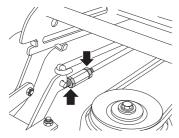
4 Screw out (extend) the stay to raise the rear edge of the cover.
