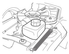
3 Fill if necessary with engine oil SAE 10W/40 (class SF–CC).
