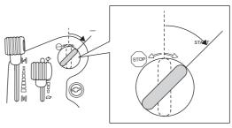
6 When the engine starts release the ignition key immediately back to neutral position.
